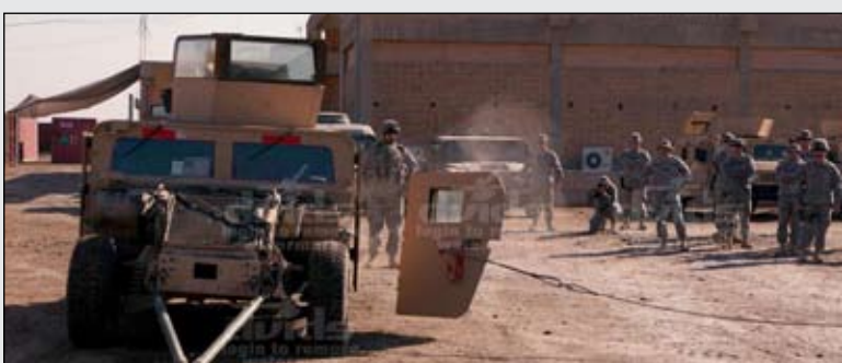
A Humvee door is pulled off using the Rat Claw, a flat steel hook developed by 2nd Brigade Combat Team, 10th Mountain Division (LI) Safety Officer Bill Del Solar. Del Solar developed the Rat Claw to aid in extraction of Soldiers from Humvees when the doors are damaged or wedged shut.
